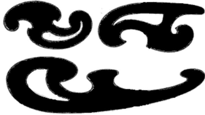
Figure 4. “A common set of [French] curves is the Burmester set displayed here. The first item is very handy for ellipses, the second very often fits large parts of hyperbolas and the third (largest) item is used most for parabolas” (Daube, 2001)
