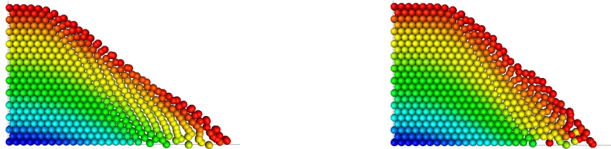
Figure 5.6: Mohr-Coulomb Dam Break – Shown on the left, \phi = 30^\circ (The actual angle of repose is approximately 36^\circ ), On the right, \phi = 60^\circ (The actual angle of repose is approximately 57^\circ )
