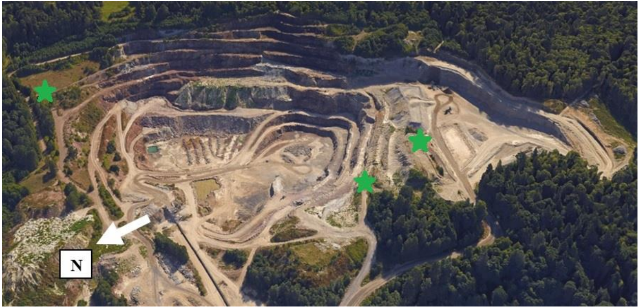
Figure 7: Aerial photograph showing the TLS scanning locations using stars (Google Earth b, 2016). The scanning locations are represented by the green stars.
