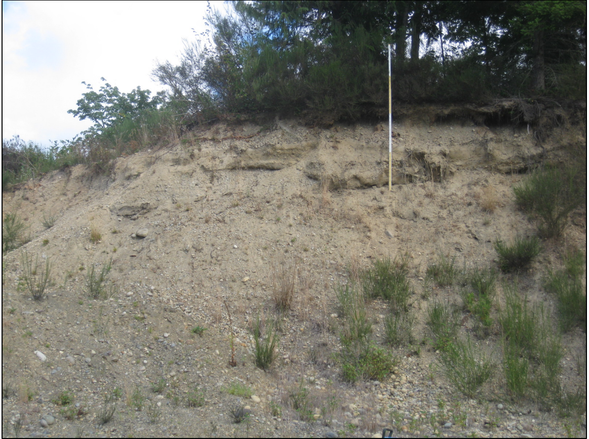
Figure 11 – EXPOSURE AT TEHALEH BACKFILL PIT #1. North-facing view of the exposure at the Tehaleh Backfill Pit #1 (site 6). Vashon till (Qvt) is present below the root layer with a sand lens about 80 cm below the root layer. The vertical reference is a telescopic stadia rod extended to 4.0 m (13.1 ft).
