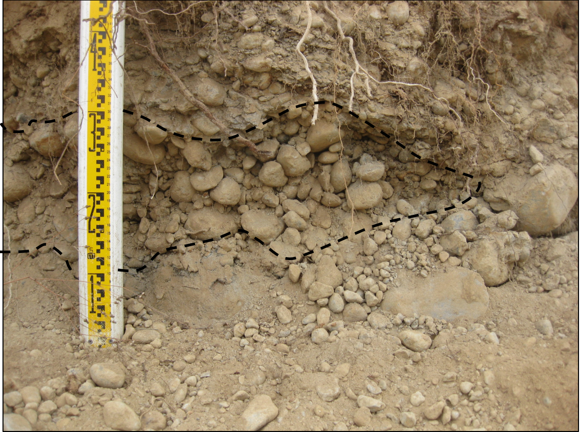
Figure 7 – GRAVEL LENS AT CORLISS GRAVEL QUARRY. Close-up view of a gravel lens in Vashon till (Qvt) at the Corliss Gravel Quarry (site 2). The dashed, black line represents the approximate boundary of the lens. The vertical scale is a stadia rod; numbered gradations represent decimeters.
