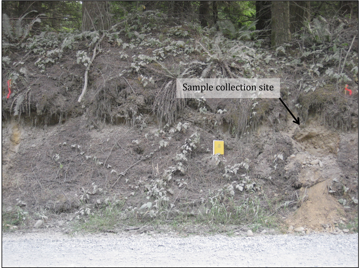
Figure 8 – WASHINGTON ROCK QUARRIES ROAD CUT. East-facing view of the road cut near the King Creek Pit operated by Washington Rock Quarries, Inc (site 3). The dugout portion is where the sample was collected, from weathered Vashon till (Qvt-w). A Rite in the Rain ® No. 540F field book is included for scale.
