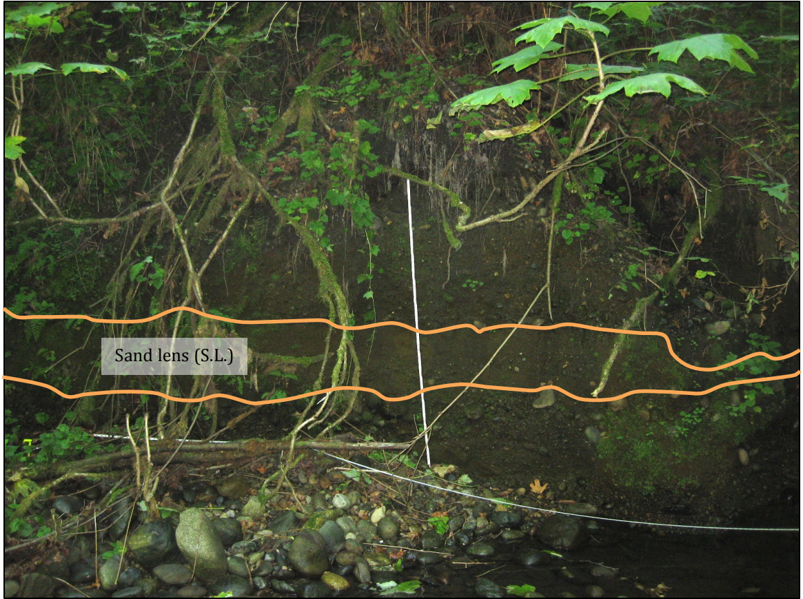
Figure 9 – SWAN CREEK EXPOSURE. East-facing view of the exposure along the right bank of Swan Creek (site 4) where a sand lens is enclosed by Vashon till (Qvt). The vertical scale is a Lufkin 6-ft. SAE folding ruler, which is fully extended.
