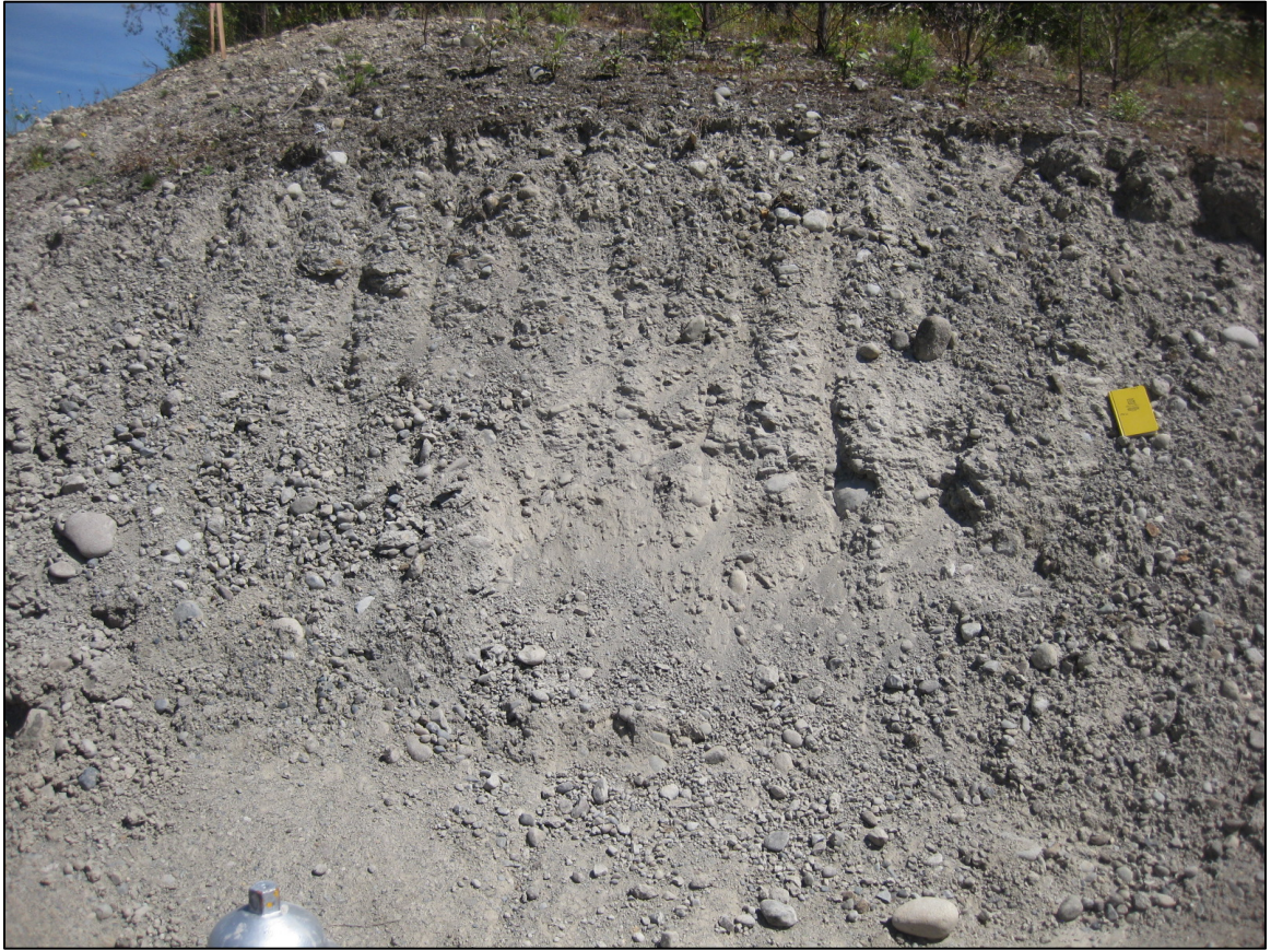
Figure 5 – COLUMBIA VISTA PHASE II ROAD-CUT. East-facing view of the road cut exposing Vashon till (Qvt) east of Overlook Dr. E in the Columbia Vista Phase II housing development (site 1). A Rite in the Rain ® No. 540F field book is included for scale.
