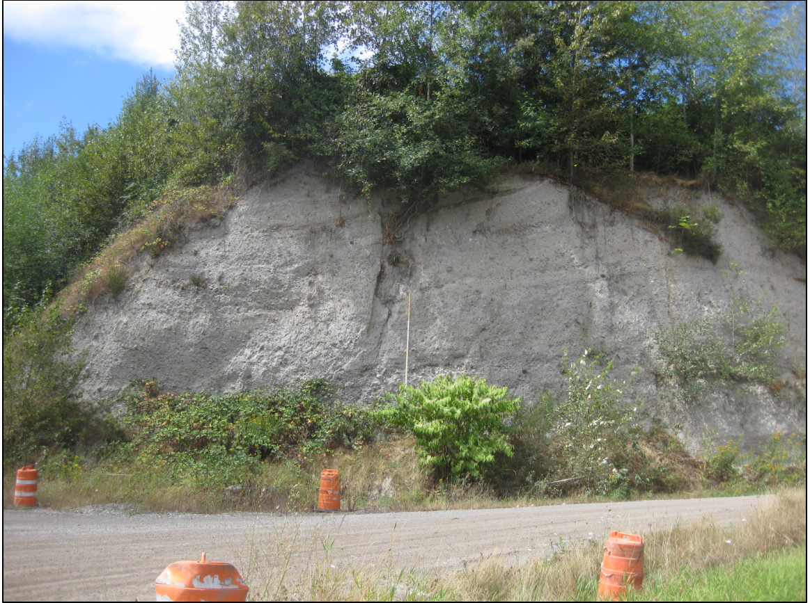
Figure 10 – EXPOSURE AT LLOYD’S SAND AND GRAVEL PIT. Northwest-facing view of the exposure at Lloyd’s Sand and Gravel Pit (site 5). The sub horizontal features are sand lenses. The vertical reference is a telescopic stadia rod extended to 5.0 m (16.4 ft.).
