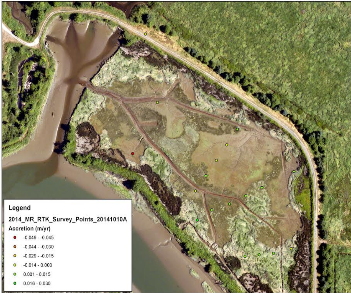
Figure 6: Map of accretion rates, reported in m/year, from RTK-GPS survey (2011-2014) in the Marysville Mitigation site Image: Jason Hall, NOAA.
