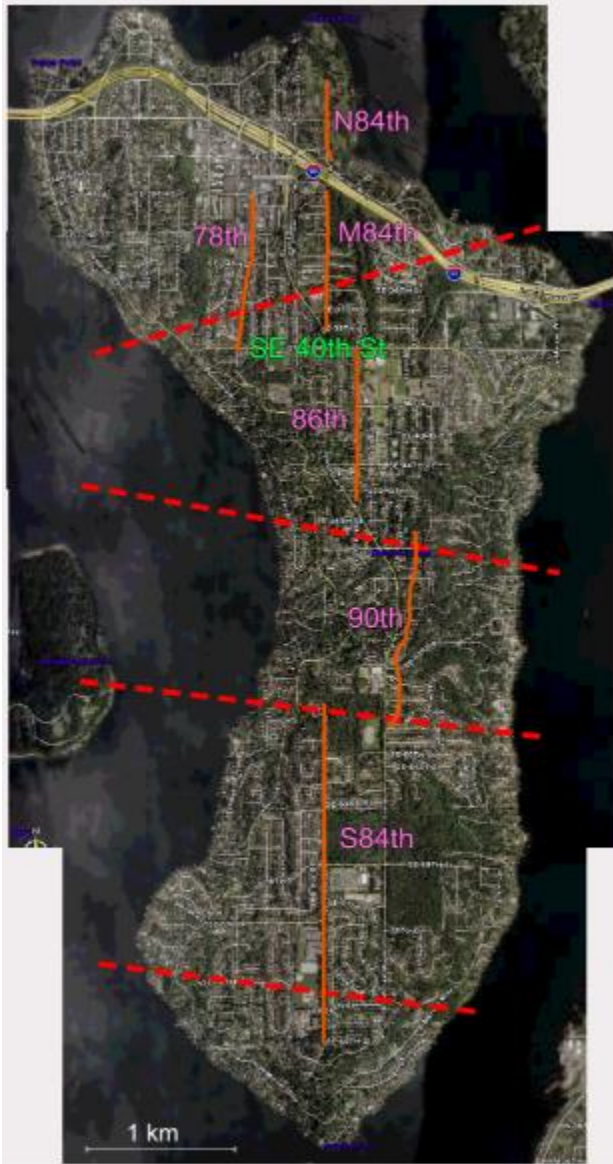
Figure 14. Map of Mercer Island showing P-wave seismic profile locations (orange lines), labeled with avenue numbers, and aeromagnetic lineaments (dashed red lines). Reproduced from Stephenson et al. (2007). The aeromagnetic lineament between 86 th Ave and 90 th Ave corresponds to the aeromagnetic lineament identified in Figure 8.
