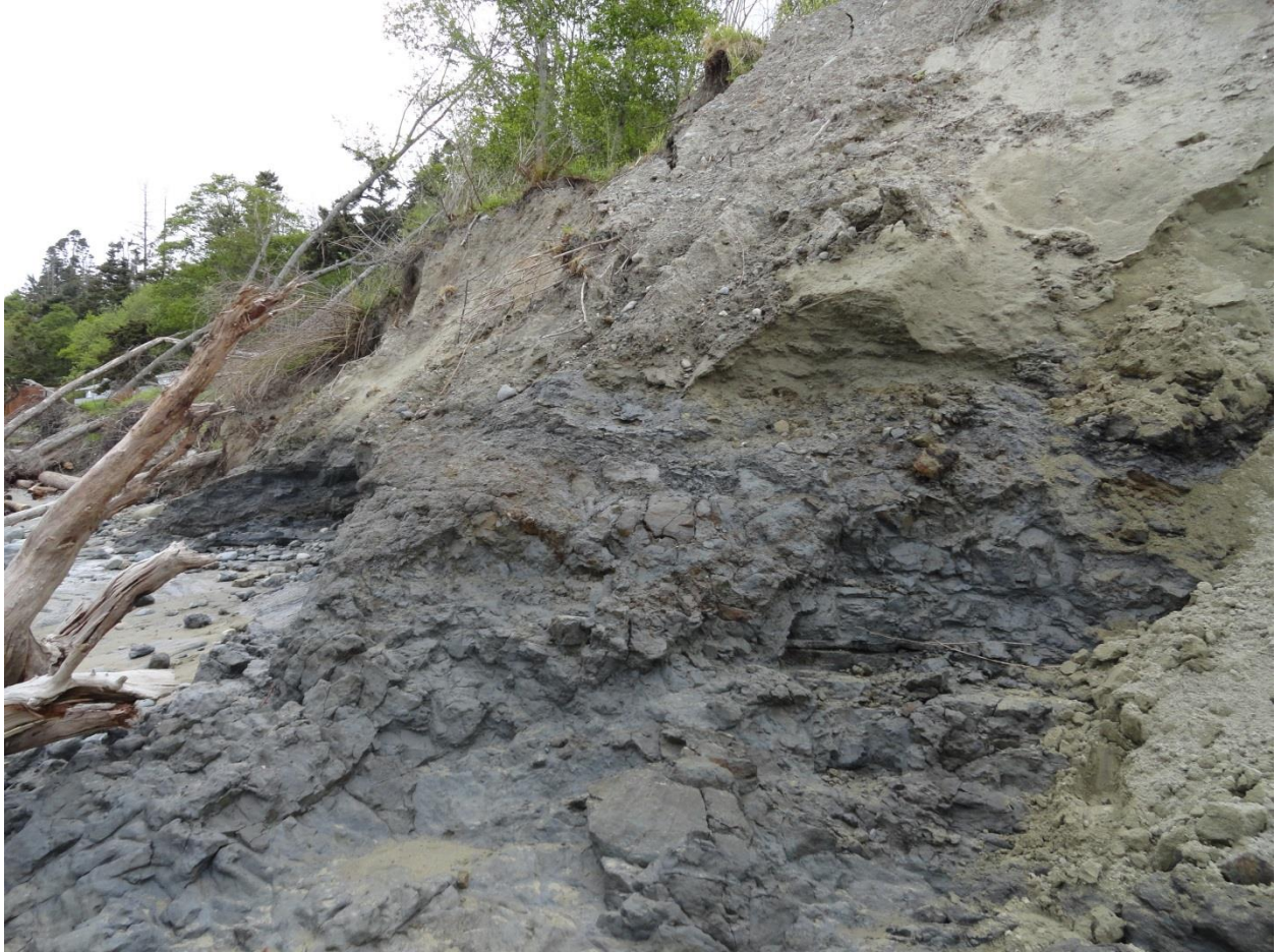
Figure 4. Clay exposed at the sampling location in the toe of the Ledgewood slide. View looks to the northeast (Photo by author, April 2014).
