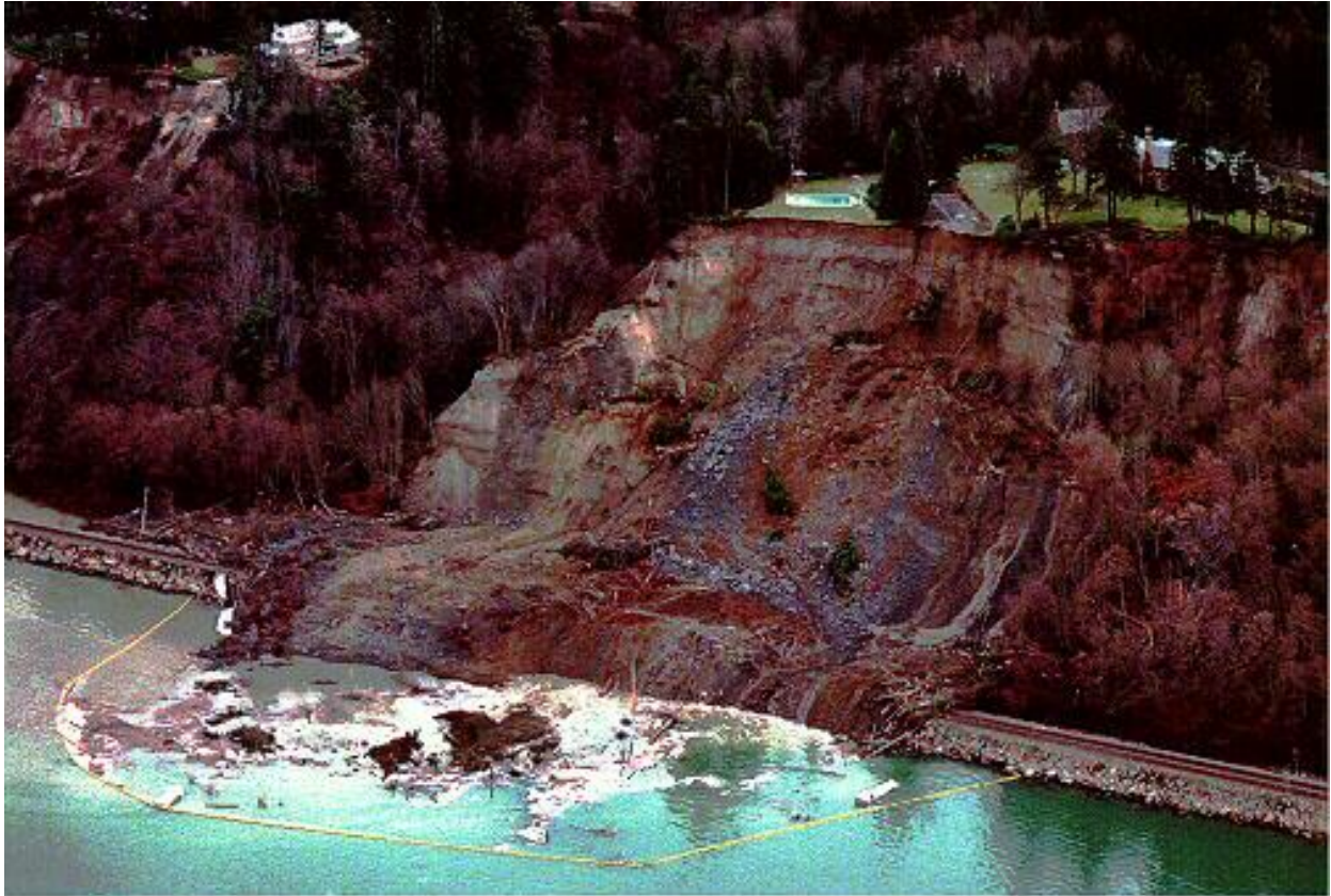
Figure 5. Oblique view of the 1997 Woodway slide looking east in the town of Woodway, WA (Baum et al., 1998). Vegetation has now recolonized the slide surface in the 17 years since this photo was taken. The sampling site is located at approximately three-quarters of the way bluff face along the north edge of the failure surface.
