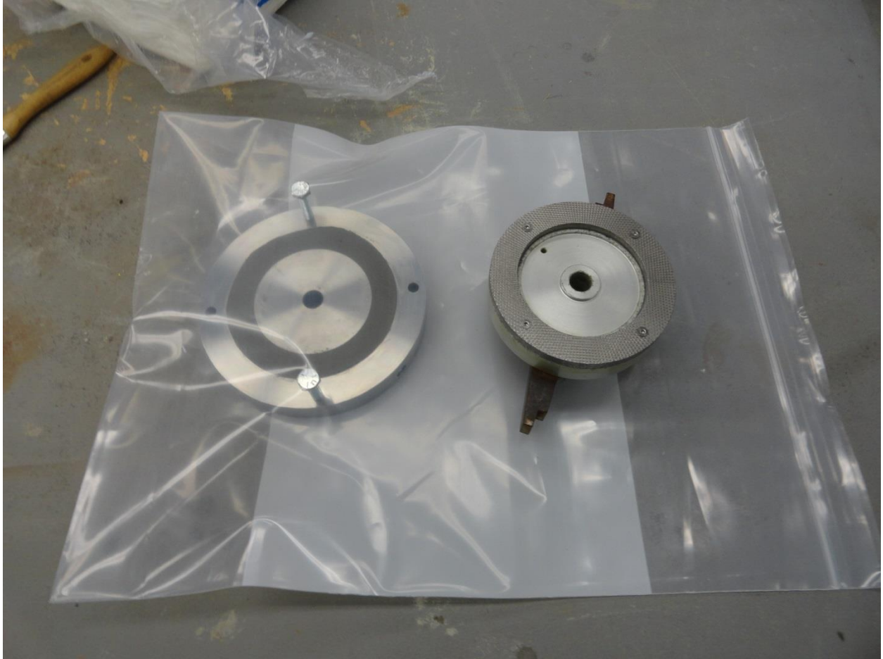
Figure 13. Photograph of the upper and lower platens of the ring shear sample vessel. The lower platen is the piece shown sealed in a plastic bag to prevent moisture loss from the clay sample loaded in the ring-shaped recess.
