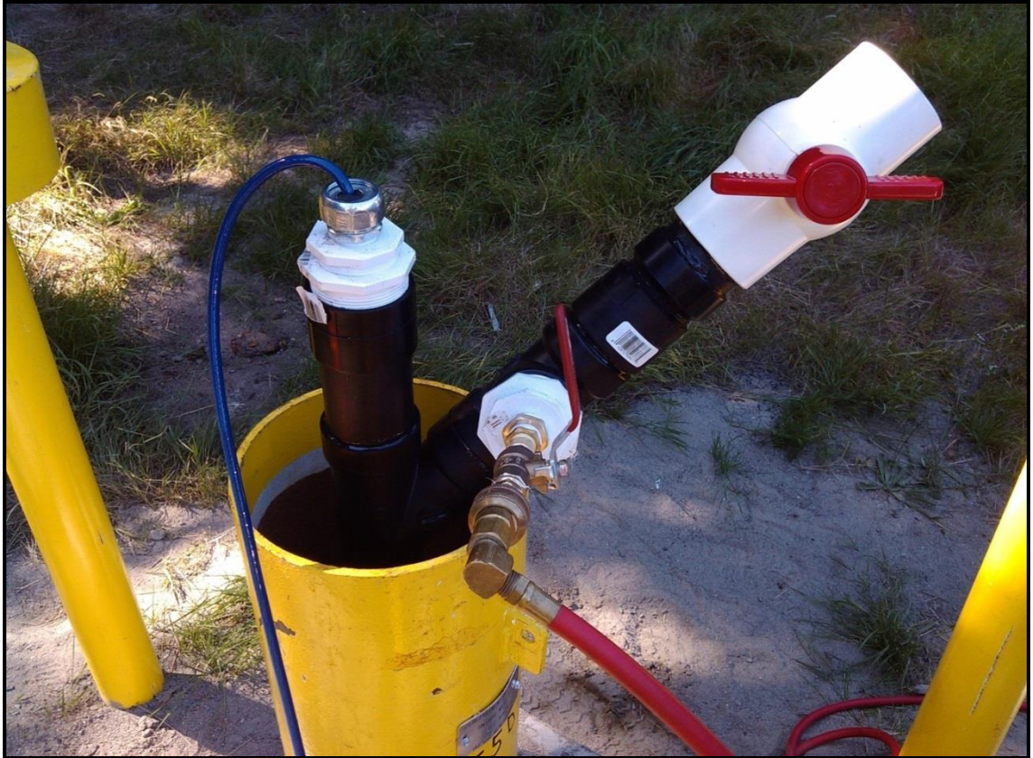
Figure 6: Pneumatic slug test device with blue transducer cable and red/white gas release valve to the right.
