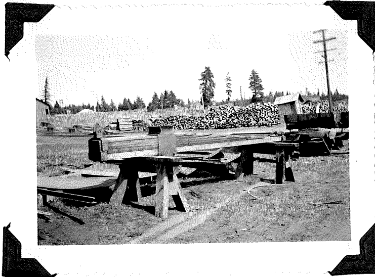
Plate II. Roslyn conveyor springboard. It is used on dips over 20° to aid the conveyor in thrusting the pans up the hill.
