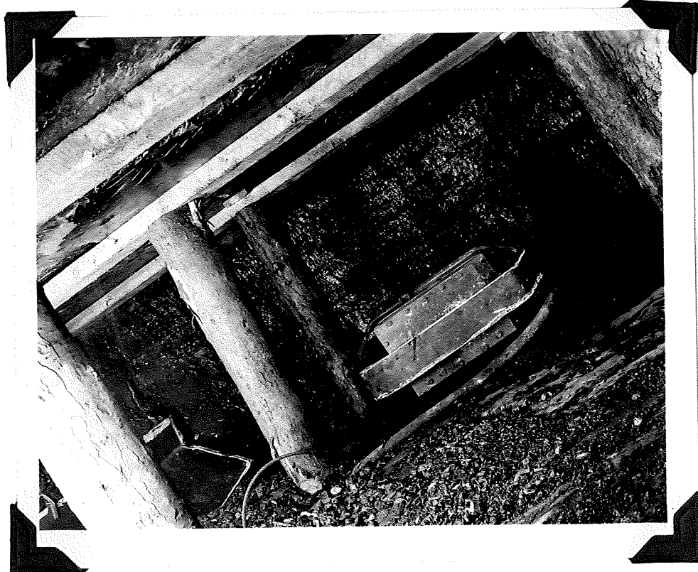
Plate VIII. Undercutter with guards in a panel room. Note the Northwestern Improvement Company guard around the sumped in "Buddy" Sullivan machine.
