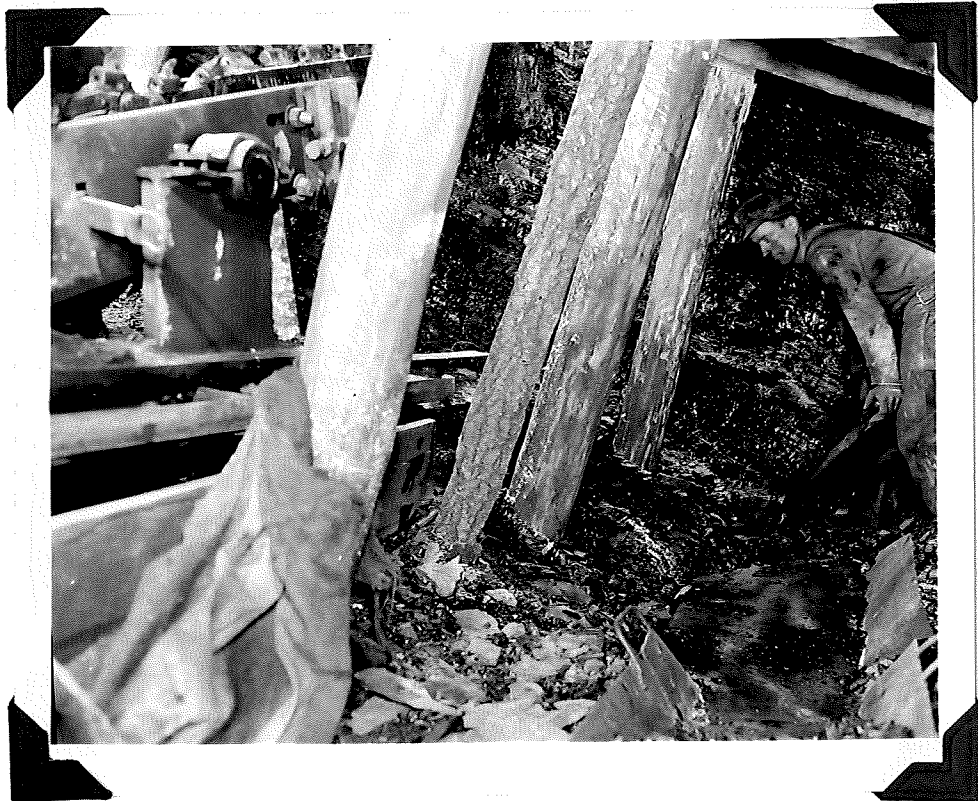
Plate VI. Shearing machine at face of the 13th East counter entry, No.5. Notice leveling-skid and the machine's hydraulic forward mechanism.
