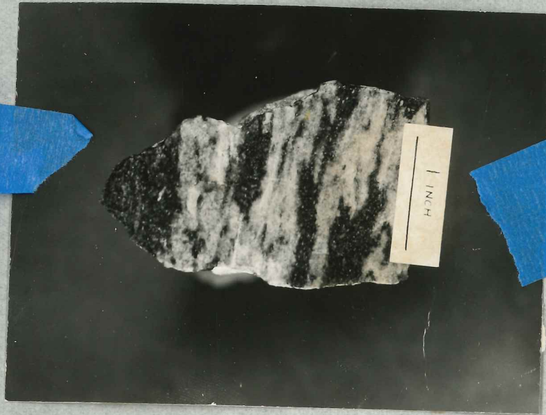
A. Banded cordierite-microcline-biotite schist showing alternations consisting mainly of diopside, calcite, and feldspars.
