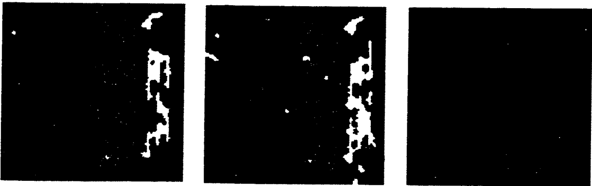
Figure 5.8 Classification maps produced by the ICM with different initializations. (a) uniform prior probability, (b) random prior probability and (c) single-color prior probability. The great differences between these maps indicate ICM's dependence on the initialization.
