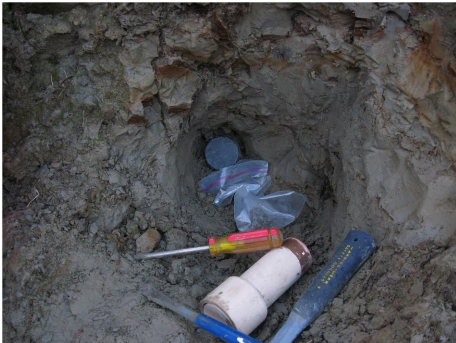
Photograph 35. Image of end cap of luminescence sampler embedded in silty sand at sample site.
