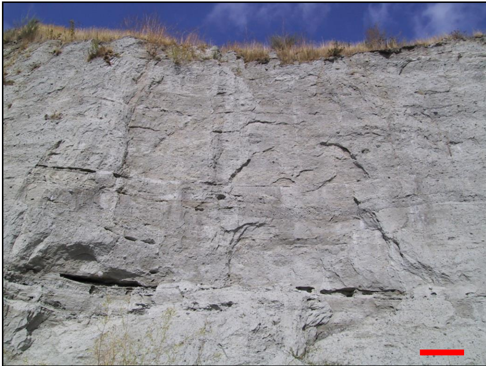
Photograph 2. Image of Vashon till at Perkins Lane, Seattle. Red bar is 2 meters in length. Voids represent where sand and groundwater had been present.
