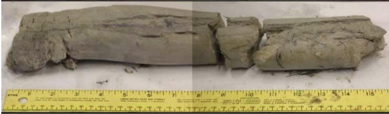
Figure 1.4. Rock core created from rock penetrator.
