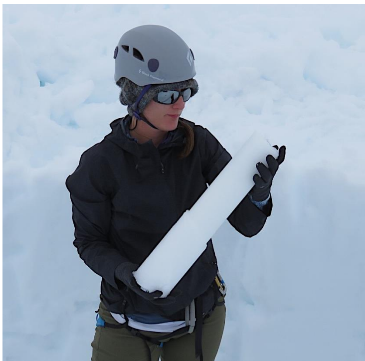
Figure 3.22. Core created by Inner Steel finless design.
