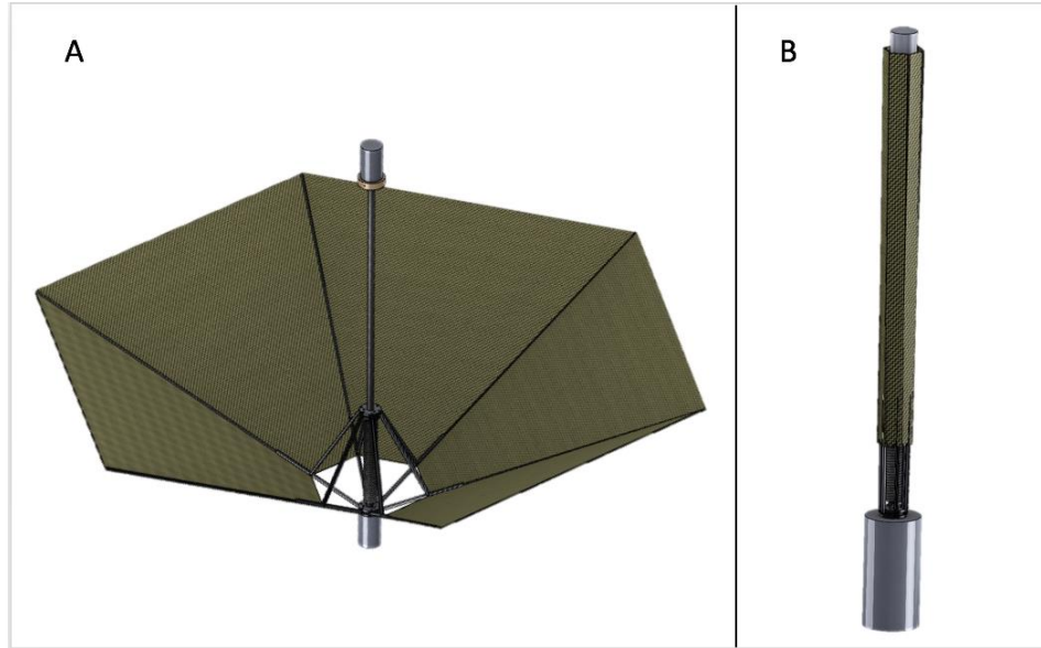
Figure 4.2. Birdie design with chute fabric. Penetrator shown attached to front, electronics to the top. A: Design mid-way open. B: Arms stowed.
