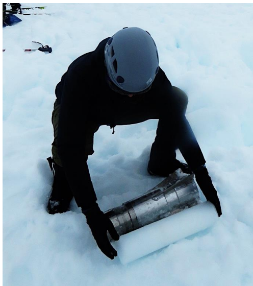
Figure 3.20. Ice core created by Long John.
