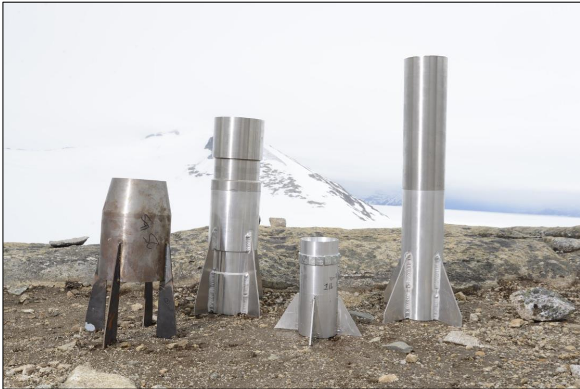
Figure 3.1. Photo of the four finned penetrators. From the left: Stumpy, Long John, Firefly, and Slim Jim.
