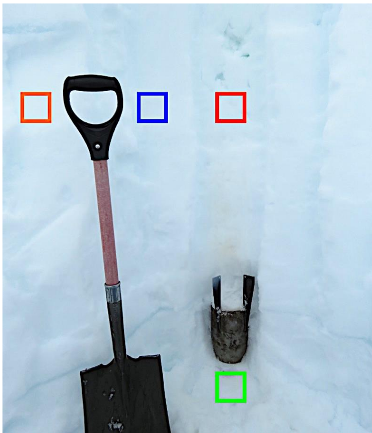
Figure 3.14. Stumpy's crater prior to removal of crater infill. Colored squares indicate where density measurements were taken: Orange – Control 1, Blue – Control 2, Red – Sample 1, Green – Sample 2.
