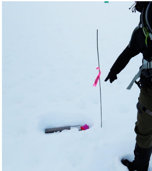
Figure 3.23. Out steel finless landing position. Due to a flat spin, the penetrator impacted on its side.
