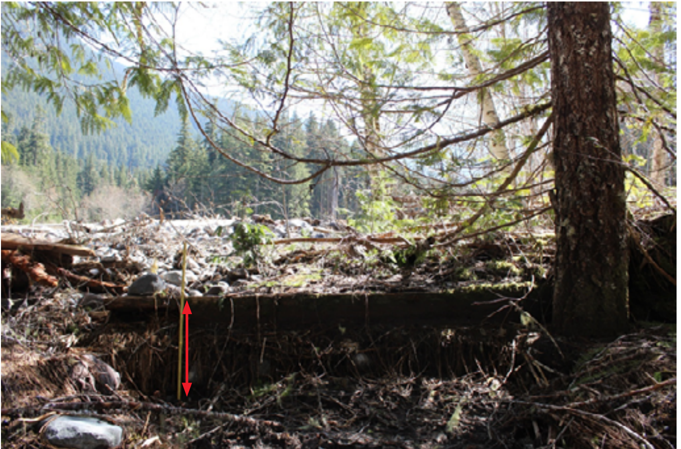
Figure 9: Double arrow line show the bed-surface elevation change at a fence jam.
