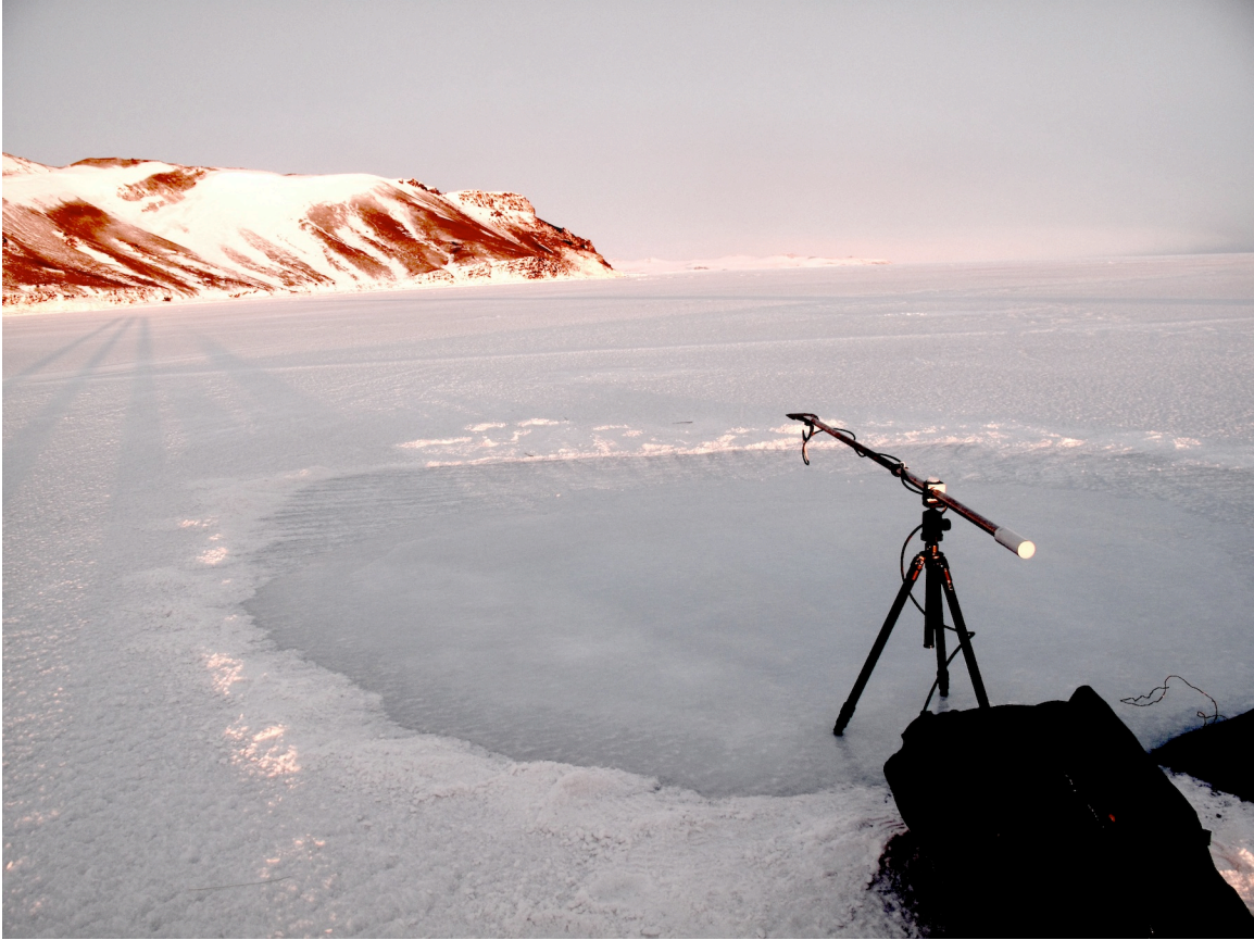
Figure 3. ASD radiometer measuring spectral albedo of sea ice in McMurdo Sound. Note cleared area, from which the 3mm crust of salty snow has been removed. 78°S, September 2009.
