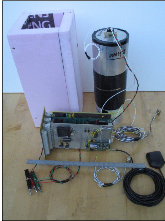
Figure 4. A photograph of the x-ray detector components: the aluminum tube (with a PMT, scintillator, high-voltage converter, and preamp inside), Styrofoam casing, and signal-processing electronics.
