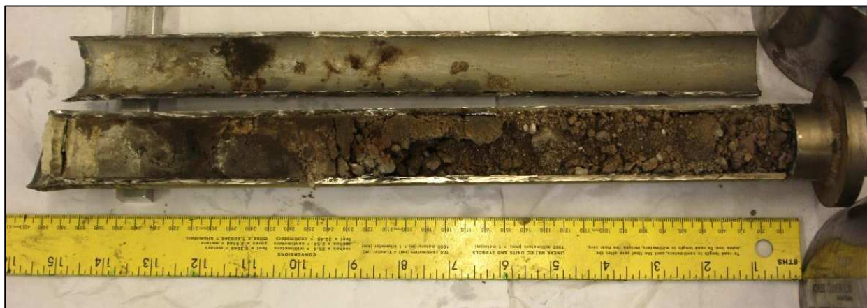
Figure 3.23. Opening the SRC revealed the stratification observed at the impact site had largely been preserved during the impact.
