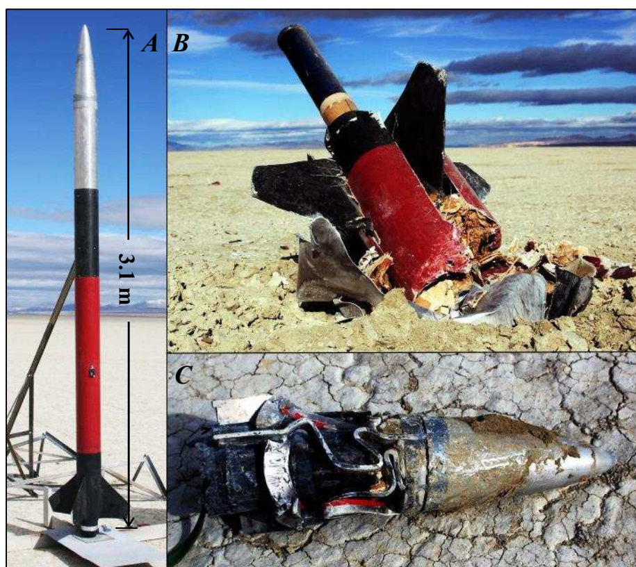
Figure 2.6. The Aluminum Rocket Prototype (ARP) inspired the design work that became the SaRSEE penetrator; (A) ARP pre-launch, (B) post-impact showing motor casing nearly ejected, (C) recovered nose cone intact with deformed stringers that absorbed the impact energy.
