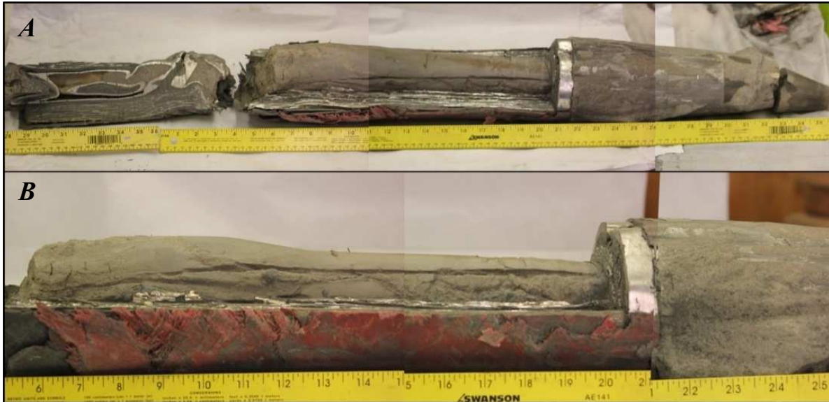
Figure 3.16. (A) The core sample was exposed after removing the encasing material; (B) note the swelling in the sample diameter near the aft end of the core, indicative of increasing pressures occurring forward of the section that experienced severe deformation.
