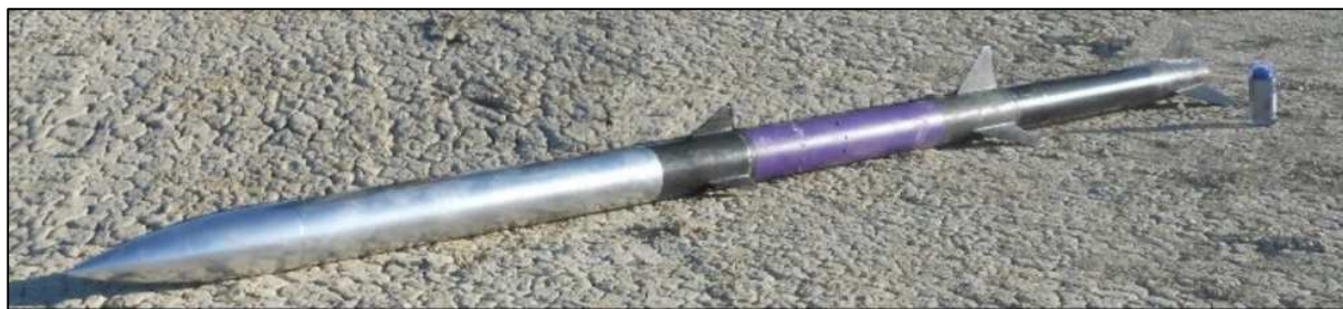
Figure 3.1. The first SaRSEE penetrator, Gravedigger 1, just prior to being loaded on the launch rail. The rocket employed an Aerotech M1850W (7,500 N-sec) in its black boost stage, and an in-line, Cesaroni N10,000 (10,347 N-sec) motor in the purple sustainer.
