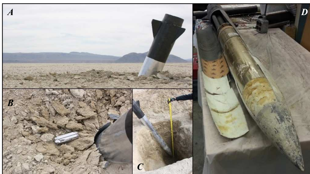
Figure 3.2. (A) During the flight of Gravedigger 1, the second stage motor casing failed during ignition when the forward enclosure sheared off. While the penetrator was blown clear, the resulting impact velocity was lower than desired ( \sim 180 m/s). (B) The impact created a clearly defined crater, with radial fractures in the playa, (C) and the penetrator embedded to a depth of 1.32 meters at an angle of \sim 30^\circ off normal. (D) Post recovery examination of Gravedigger 1 revealed the impact resulted in almost no internal damage to the penetrator, but the impact velocity was too low to open the feed ports that had been covered with carbon fiber, so no sample was collected.
