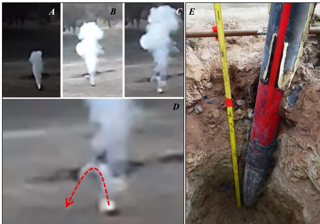
Figure 3.21. (A)(B)(C)(D) Still frames from a video of the impact show the SRC entraining part of the smoke plume as it ejected at about 10 m/s, coming to rest about 2 m from the embedded penetrator. (E) The penetrator embedded to a depth of 1.27 m through stratified layers of soil, clay, and talc.
