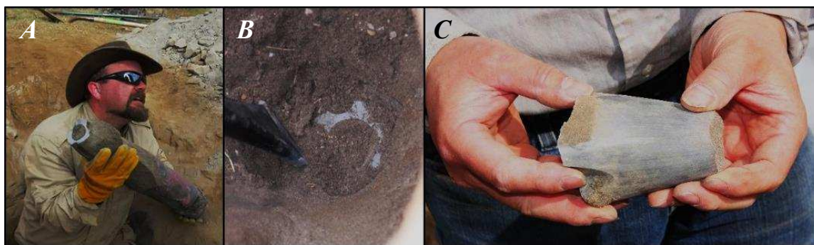
Figure 3.12. (A) The removal of the main body of the penetrator; (B) forces during the impact resulted in a brittle failure 7.6 cm aft of the front of the steel tip, leaving the separated portion embedded in the sandstone after the main body of the penetrator was recovered; (C) the recovered steel tip.
