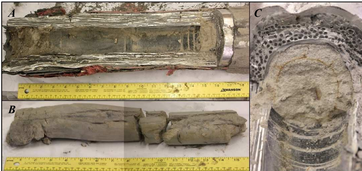
Figure 3.17. (A) The feed chimney after the removal of the core sample; (B) the sample core was very solid, and required fracturing it in multiple locations to remove it from the chimney; (C) sample material in the nose cone was left in place given the difficulty in removing it intact.
