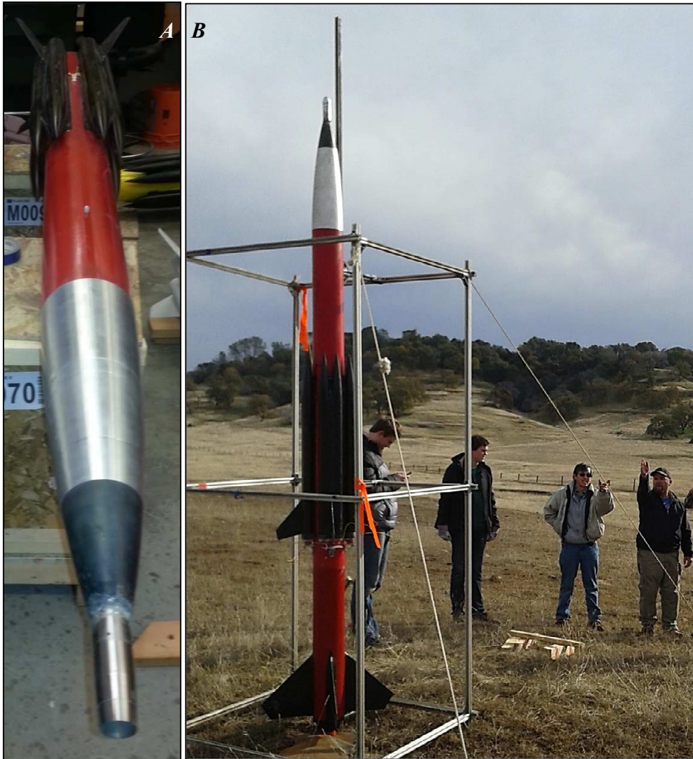
Figure 3.19. (A) The epoxied SRC with its tip in front of the main nose cone and (B) the penetrator system ready for flight.
