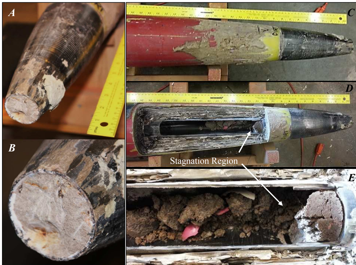
Figure 3.5. (A & B) The center-bored feed port, steel nose cone sustained no significant damage; (C) measurements made through the aft of the penetrator suggested material flow had stagnated around 0.33 meters after impact; (D) the penetrator in cross-section, showing the stagnated material inside the feed chimney; (E) close-up of the stagnation point with remnants of the feed port cover (pink shell fragments) mixed in the ejecta.
