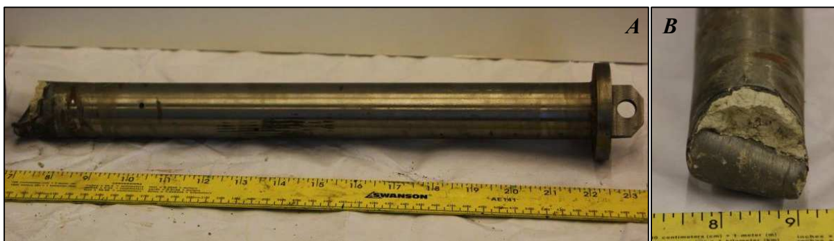
Figure 3.22. (A) The recovered SRC showed no deformation along its length and (B) slotted tabs at the feed port folded over during impact to partially close the SRC.
