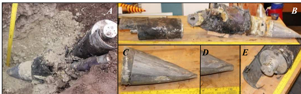
Figure 3.8. (A) The penetrator embedded to a depth of \sim 0.9 meters, but was deflected off a straight trajectory when it struck a piece of quartzite; (B) the deflection resulted in massive deformation of the penetrator that separated the body at unreinforced seams in the energy absorbing core material, and prevented sample material from reaching the SRC; (C) the aluminum nose cone experienced some deformation during the impact, although the feed ports remained open; (D) the contact point where the nose cone encountered the quartzite; (E) the SRC remained intact, but warping in the airframe resulted in binding.
